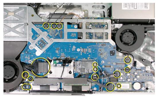
Replace the machine screw first; then replace the self-tapping screws.
